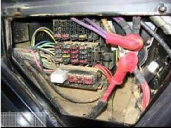
A photograph showing the interior of a fuse box. The box is open, revealing a complex arrangement of electrical components. In the center, there is a fuse block with several fuses. To the right, there are two prominent red components, possibly relays or solenoids, connected to thick red wires. Various other colored wires (yellow, green, blue, purple) are visible, some bundled together. The background shows the metal structure of the fuse box and some internal wiring harnesses. |
