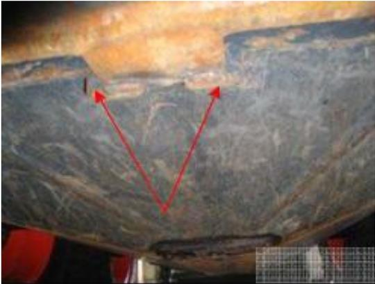
A close-up photograph of a metal surface, likely the underside of a vehicle. Two small, circular drainage holes are visible, each highlighted by a red arrow. The surface appears to be covered in a layer of dirt or biosecurity risk material, making the holes difficult to see.             |
