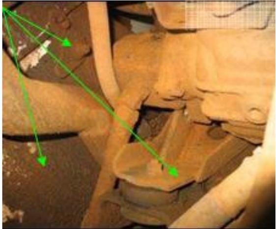
A photograph showing the underside of the vehicle cabin. Several green arrows point to various surfaces, including metal plates and structural components, which are heavily covered with a thick, brownish, crumbly residue, illustrating the amount of biosecurity risk material that can accumulate. |
