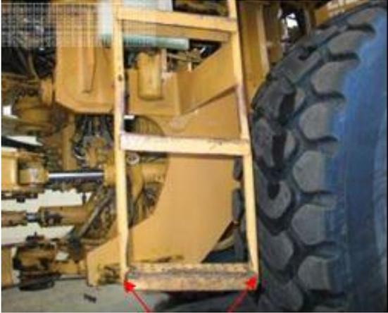
A photograph of a yellow ladder leading up to the cabin of a wheel loader. Two red arrows point to the ends of the ladder's rungs, which are open-ended tubes. These areas are highlighted as needing to be flushed for biosecurity.                                                                  |
