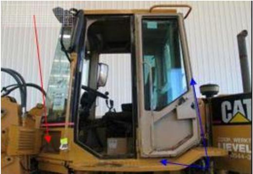
A side-view photograph of a yellow wheel loader cabin. A red arrow points to a removed panel on the side. Blue arrows point to the removed rubber seals on the door and side panels. |
