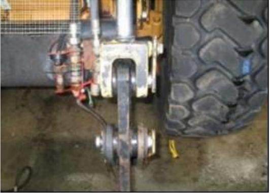
A close-up photograph of the bucket arm pivot points on a wheel loader. The image shows the metal components, including the bucket arm, the pivot pin, and the hydraulic cylinder. A large, treaded tire is visible in the background. |
