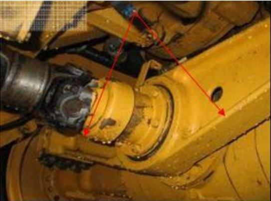
A close-up photograph of a yellow metal sway bar assembly. Two red arrows point to horizontal ledges on the bar, one pointing to a ledge on the back and one pointing to a ledge on the front. The assembly is part of a larger mechanical structure. |
