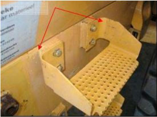
A close-up photograph of a yellow machine footprint, which is a textured plastic plate used for walking on heavy machinery. Two red arrows point to the underside of the footprint, highlighting areas that are difficult to clean and may harbor contaminants.                                        |
