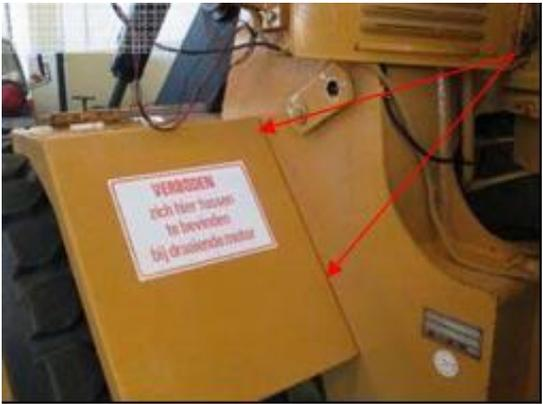
A photograph of a yellow wheel loader's wheel arch. A white warning sign with red text is attached to the arch. Two red arrows point to the seam between the arch and the wheel hub, indicating where to flush for cleanliness. The sign reads: "VERBODEN zich hier tussen te bevinden bij draaiende motor" (Prohibited from being in this area when the motor is running). |
