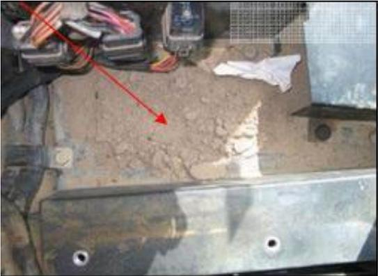
A close-up photograph of a removed joystick control panel. A red arrow points to a surface that is heavily contaminated with a light-colored, fibrous material. The panel is resting on a metal surface.                                                                                                                                                                                                    |
