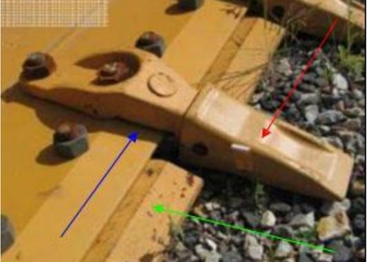
A close-up photograph of the cutting teeth and blade on a bucket. A red arrow points to a cutting tooth, a green arrow points to the cutting blade, and a blue arrow points to a small recessed area on the blade.                   |
