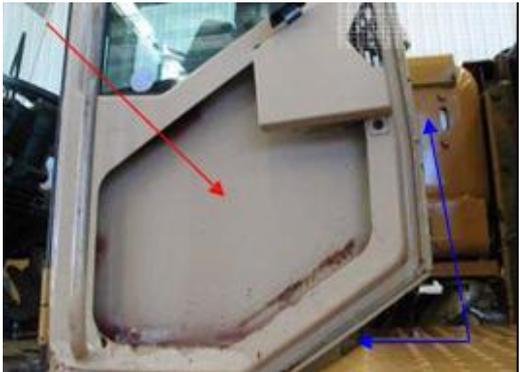
A close-up photograph of the interior of a door. A red arrow points to the removed internal panelling. Blue arrows point to the removed rubber seals on the door frame.             |
