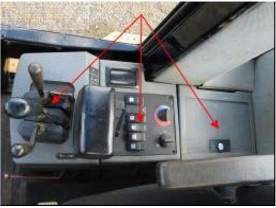
A close-up photograph of the joystick control panels in the cab. Two red arrows point to the internal surfaces of the joystick bases. Another red arrow points to a panel on the right side of the control area. The panels are grey and have various buttons and switches.                                                                                                                                  |
