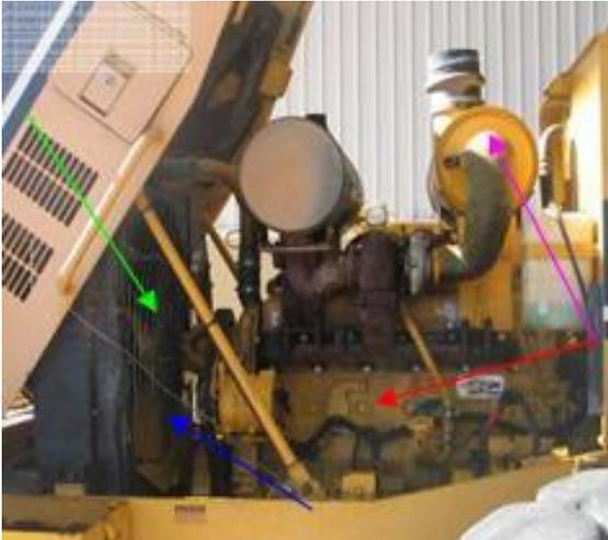
A wide-angle photograph of the engine block and radiator. A blue arrow points to the internal radiator grill. A green arrow points to the harmonic balancers. A purple arrow points to the air-filter. A red arrow points to the side of the engine block. |
