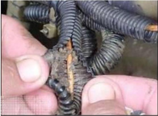
A close-up photograph showing a person's hands holding a black, braided wiring harness. A significant hole has been made in the outer sheath of the cable, exposing the internal copper wires. The person's fingers are positioned to show the extent of the damage.                                                                     |
