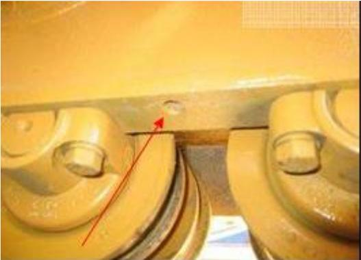
A close-up photograph of a yellow metal rock guard assembly on a Caterpillar dozer. A red arrow points to a specific location on the assembly where a bolt has been removed, providing access to a hollow section above.                                                                                             |
