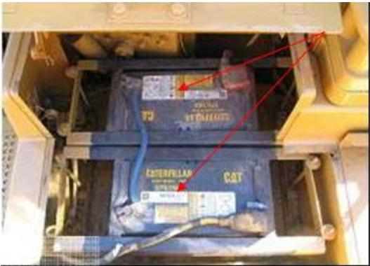
A photograph showing the interior of a Caterpillar dozer's battery compartment. Several blue batteries are visible, secured by metal tie-downs. Red arrows point to the tie-down points, indicating where they should be loosened for cleaning and inspection. The batteries have "CATERPILLAR" and "CAT" branding. |
