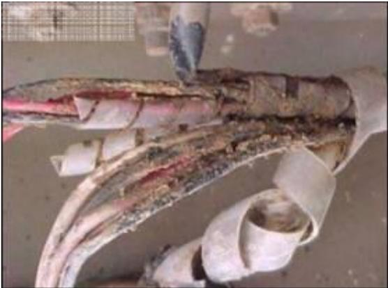
A photograph showing a bundle of hydraulic hoses wrapped in white tape. The tape is peeling away, revealing a dark, greasy residue and some red markings on the underlying hoses, indicating contamination or damage.                                                                                                                   |
