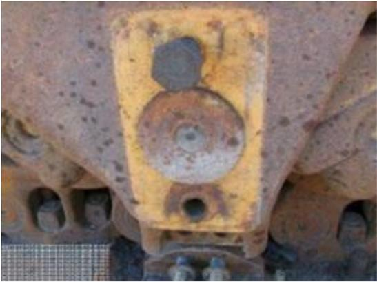
A close-up photograph of a bearing cover on a dozer track. The cover is a circular, concave metal component, heavily rusted and discolored. It is mounted on a larger metal frame.                      |
