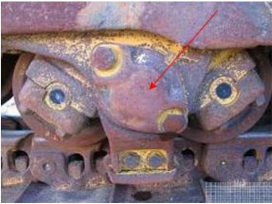
A photograph showing a bearing cover on a D8 dozer track. A red arrow points to the cover, which is still attached to the track. The cover is heavily rusted and discolored.                           |
