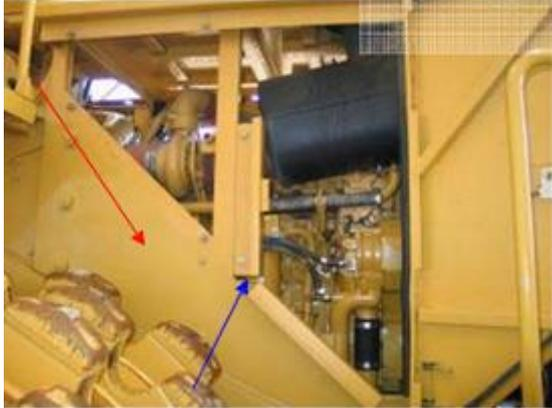
A photograph showing the interior of a yellow engine housing. A red arrow points to a non-affixed panel, and a blue arrow points to a hollow framework structure. |
