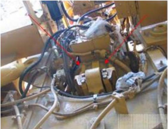
A photograph of the engine block area of a compactor with the cabin removed. Red arrows point to the bell housing, which has a complex, undulating surface. The area is cluttered with hoses, wires, and other mechanical parts. |
