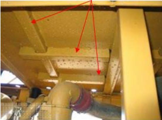
A photograph showing the underside of the engine housing. Red arrows point to hollow, open-ended support channels.                                               |
