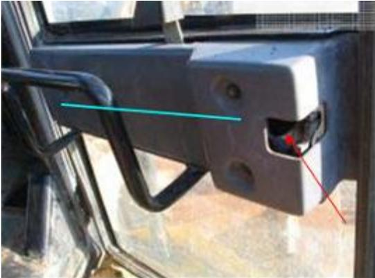
A close-up photograph of a door latch mechanism. A red arrow points to a small, dark, hollow opening in the metal structure, which requires internal cleaning for biosecurity.                            |
