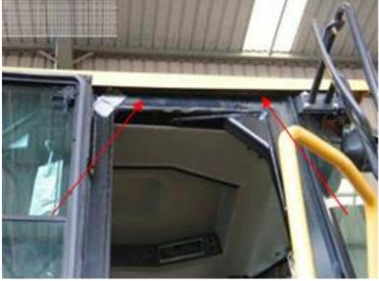
A photograph showing the top of the cabin and the Roll Over Protection System (ROPS). Two red arrows point to a narrow gap or recess between the cabin roof and the ROPS structure.                      |
