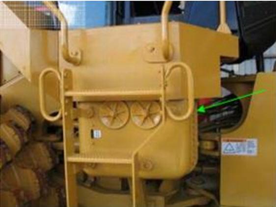
A photograph of the yellow oil tank located under the operator's cabin. The tank is cylindrical and has several access points. A green arrow points to a specific access point on the rear side of the tank, which is noted as being difficult to reach.               |
