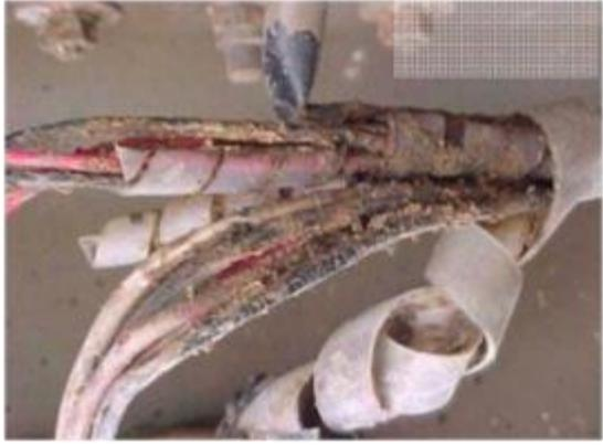
A close-up photograph of a wiring harness. A blue arrow points to a section of the harness where there is visible dirt and debris, highlighting the need for internal cleaning.                           |
