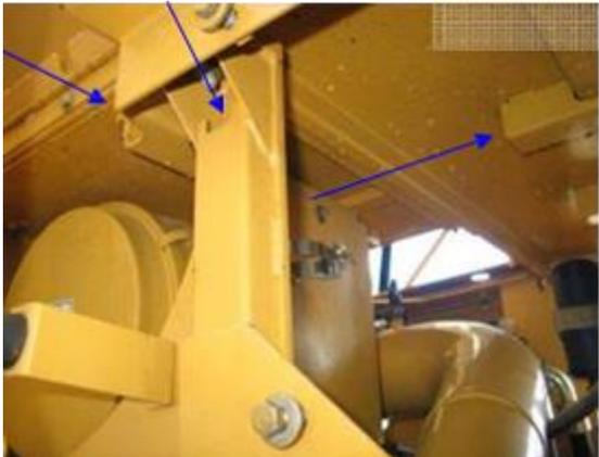
A photograph showing the hollow support framework under the engine cover. Blue arrows point to the framework.                                                   |
