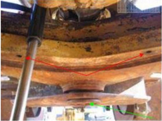
A photograph showing the underside of a compactor's chassis. A vertical metal rod is visible on the left. A red double-headed arrow points to a narrow, V-shaped hollow channel between two curved metal plates. A green arrow points to a pivot point on a lower plate. |
