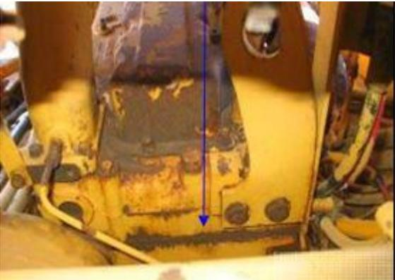
A photograph showing the topside of the engine block as seen from below the floorpan. A blue arrow points to the rear end of the block, indicating it can be accessed for cleaning and inspection. |
