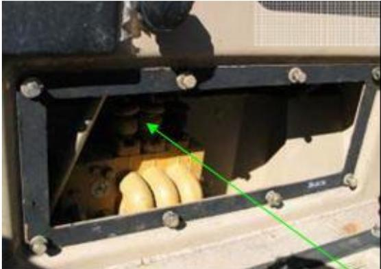
A photograph showing the internal view of the right-hand joystick control panel. The panel is removed, revealing a complex arrangement of hydraulic hoses and mechanical components. A green arrow points to a specific area within the internal structure, likely indicating a point of interest for cleaning or inspection. |
