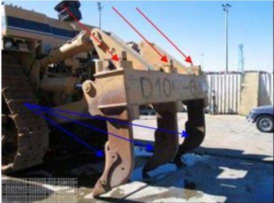
A photograph of a dozer blade assembly. Red arrows point to recesses between the cradle and tynes. Blue arrows point to wear plates on the tynes. |
