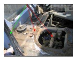
An illustration of the fuel cell under the seat. In some instances, the cabin will require unbolting and lifting to allow cleaning and inspection access to the topside of the fuel cell and hydraulic hoses (currently not in view). The bands around the tank (red arrows) need to be loosened off and flushed to remove any contaminants.
