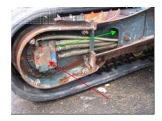
Rock guards would be rare on mini excavators however if present, these must be removed to allow cleaning and inspection access to the inside track frame. The blue arrows highlighting the frame above the rock guards may be a hollow channel or at least an internal ledge, which requires inspection.
