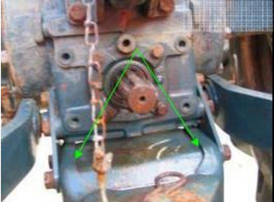
A close-up photograph of a blue tractor component. Two green arrows point to small, recessed areas on the metal surface, which are intended to be flushed for cleanliness.                                              |
