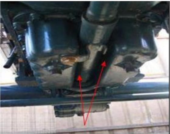
A photograph of an unusual sump design. The steering shaft divides the sump through the center. Red arrows point to the areas where the shaft meets the sump, indicating potential biosecurity risk material accumulation.     |
