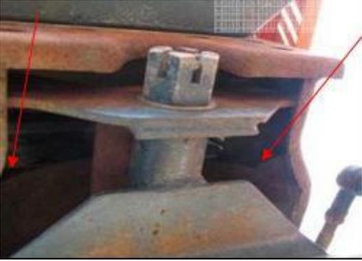
A close-up photograph of a chassis rail. Two red arrows point to hollow cavities or recessed areas on the underside of the rail, near the front nose of the tractor. |
