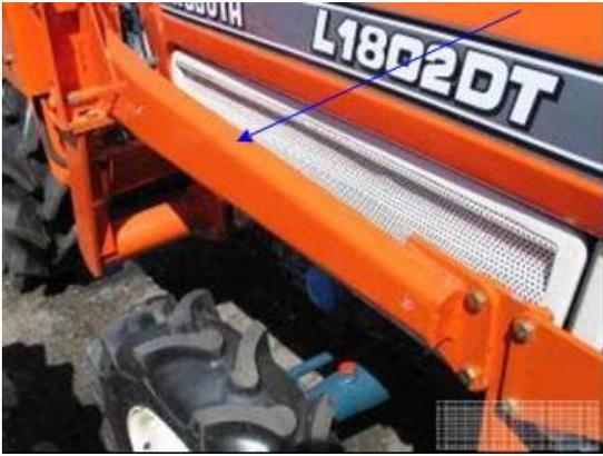
A close-up photograph of an orange tractor's push arm. A blue arrow points to the arm. The tractor's body has the text 'L1802DT' visible. A small grid pattern is in the bottom right corner. |
