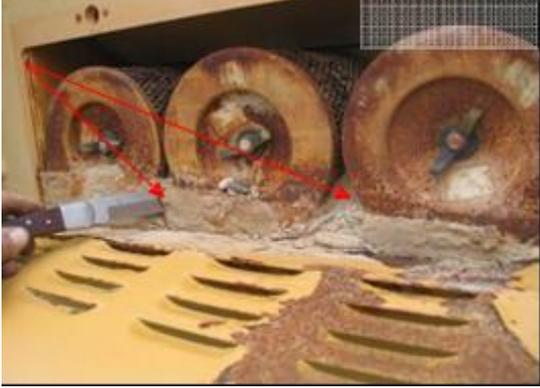
A close-up photograph of three circular air filters mounted in a row. Red arrows point to the filters, highlighting the area where BRM (Biosecurity Risk Material) is likely to accumulate. The filters are surrounded by a mesh screen and are positioned above a yellow metal grate. |
