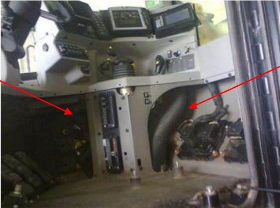
A close-up photograph of the joystick control panel area. Two red arrows point to the gaps where non-affixed panels have been removed, providing access to the internal components like the air conditioning and steering unit. The seat and floor mats are also absent.       |
