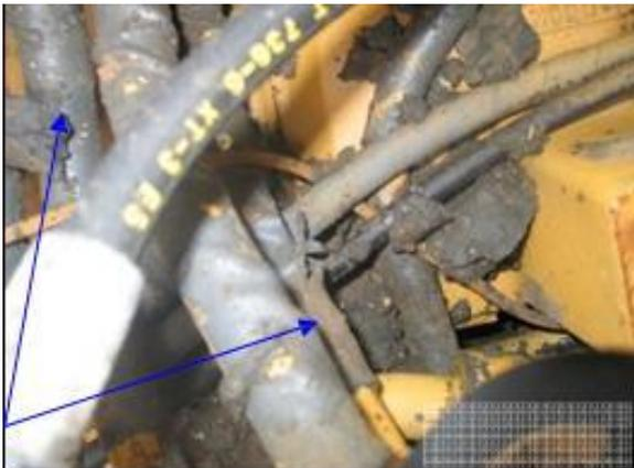
A close-up photograph of hydraulic hoses. Two blue arrows point to areas where BRM (Biosafety Residue Material) is visible on the hoses. The hoses are surrounded by other mechanical parts and grease.           |
