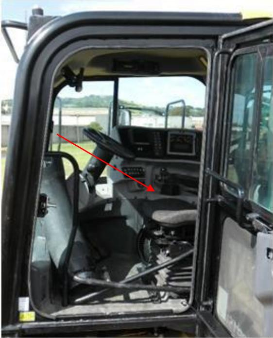
A photograph showing the interior of a machine cabin from an open door. A red arrow points to the joystick control panel located on the right side of the operator's seat. The cabin contains a steering wheel, a dashboard with a digital display, and various control levers. |
