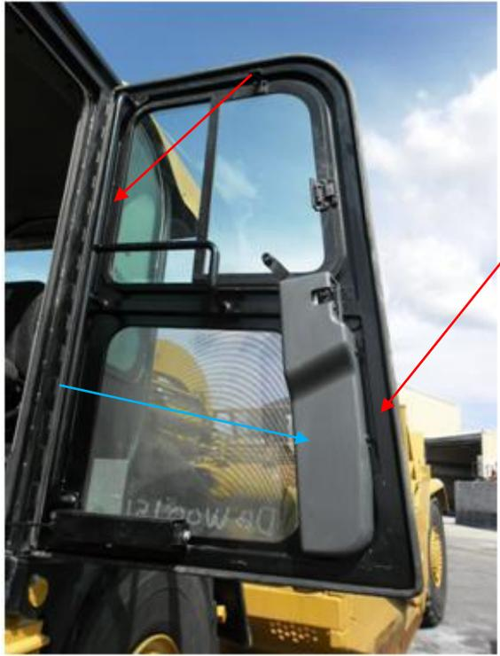
An exterior photograph of a yellow machine's door. Two red arrows point to the rubber seals at the top and bottom of the door frame. A blue arrow points to the internal door lining. The machine is parked outdoors under a blue sky with clouds. |
