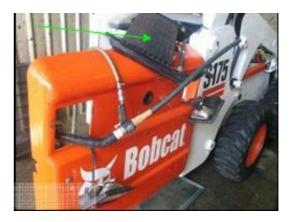
Another example of skid steer engine block. The battery has been removed (yellow arrow) and all non-affixed components have been removed, allowing greater cleaning and inspection access.
