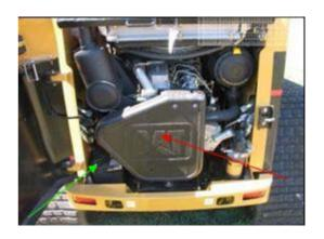
The lights have been removed from the rear door for cleaning and inspection. All foam insulation inside the door (reverse side) must be flushed to verify cleanliness. The radiator core (green arrow) has also been unbolted to facilitate the cleaning and inspection process.
