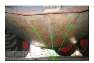
This underbelly is from a tracked model skid steer loader (red arrow). On this model there are several non-affixed panels that can be easily removed, allowing cleaning and inspection access as well as providing exit points for biosecurity risk material under the cabin.
