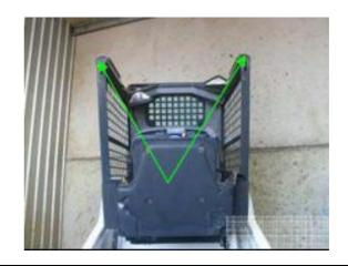
On other models, the box section under the seat may be accessible via small nonaffixed plates like the one illustrated by the blue arrow. The rubber seat shroud (green arrow) must be thoroughly cleaned both inside and out.
