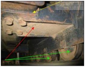
Another view of the rear axle however the main focus is on the small drainage holes (green arrows) located halfway along the bottom chassis. Small non-affixed cover plates have been removed, allowing flushing and inspection access.
