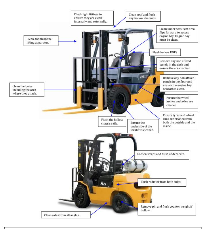
The most common type of contamination found on forklifts is contaminated grease. Grease itself is not a biosecurity concern but after time it will attract biosecurity risk material such as soil, seeds and plant material. Once grease becomes contaminated it must be removed to meet the Department of Agriculture and Water Resources standards.
