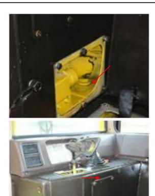
These pictures illustrate the various compartments found under the seat and around the seat. All non-affixed panels have been removed, allowing access for cleaning and inspection. These areas sometimes have ledges inside which can harbor biosecurity risk material and need to be thoroughly inspected. Care must be taken when inspecting electronics in this area.
