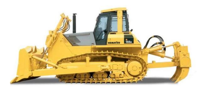
Landscape shot of a typical Komatsu Dozer. Structurally, the larger dozers (D51 to D375) are basically the same except for small variations and obviously size differences. The smaller Komatsu Dozers (D21 to D39) are a different style as shown below.
