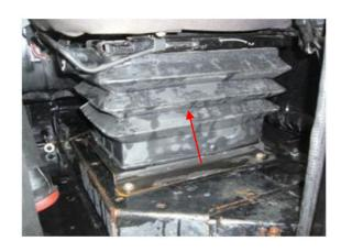
These pictures are examples of compartments behind the seat that must be opened and inspected. Look and check for cabin air filters and hollow areas behind these filters.
