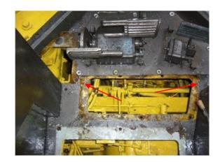
The seat has to be removed to allow access to the top of the transmission and to any compartments that are behind the seat.
